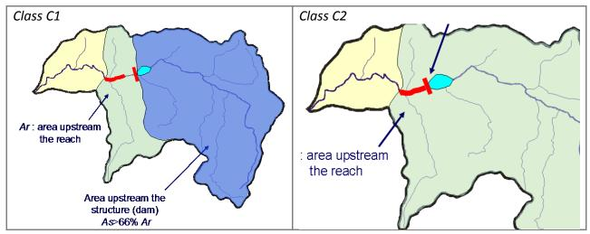
Figure A3.39 Upstream alteration of sediment discharges (2). *Class C1*: dam (T1) with a drainage area > 66% of the area upstream from the reach (left). *Class C2*: dam (T1) at the upstream limit of the reach (right).
