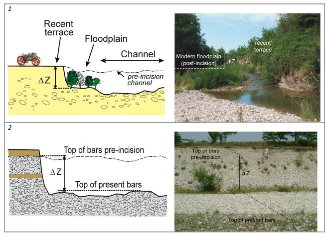
Figure A3. 67 Estimation of the amount of incision based on differences in elevation among surfaces. (1) Measurement of difference in elevation ( $\Delta z$ ) between modern floodplain and recent terrace (pre- incision floodplain); (2) measurement of difference in elevation between the top of gravel on an eroding bank (corresponding to the top of bars before incision) and top of present channel bars.
